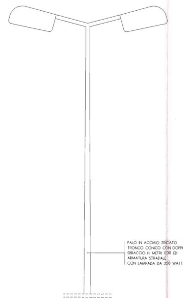
PALO IN ACCIAIO ZINCATO TRONCO CONICO CON DOPPIO BRACCIO H. METRI 1000 ED ARMATURA STRADALE CON LAMPADA DA 250 WATT.
